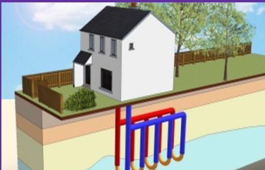
*Illustration of Vertical GSHP system, thanks to the British Geological Survey*
